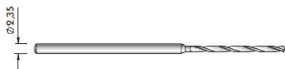
Drill \varnothing 1,2 mm, 44/10 mm (stainless steel)
